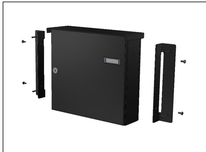
Figure 28 - Mounting the mounting bracket on the letterbox
