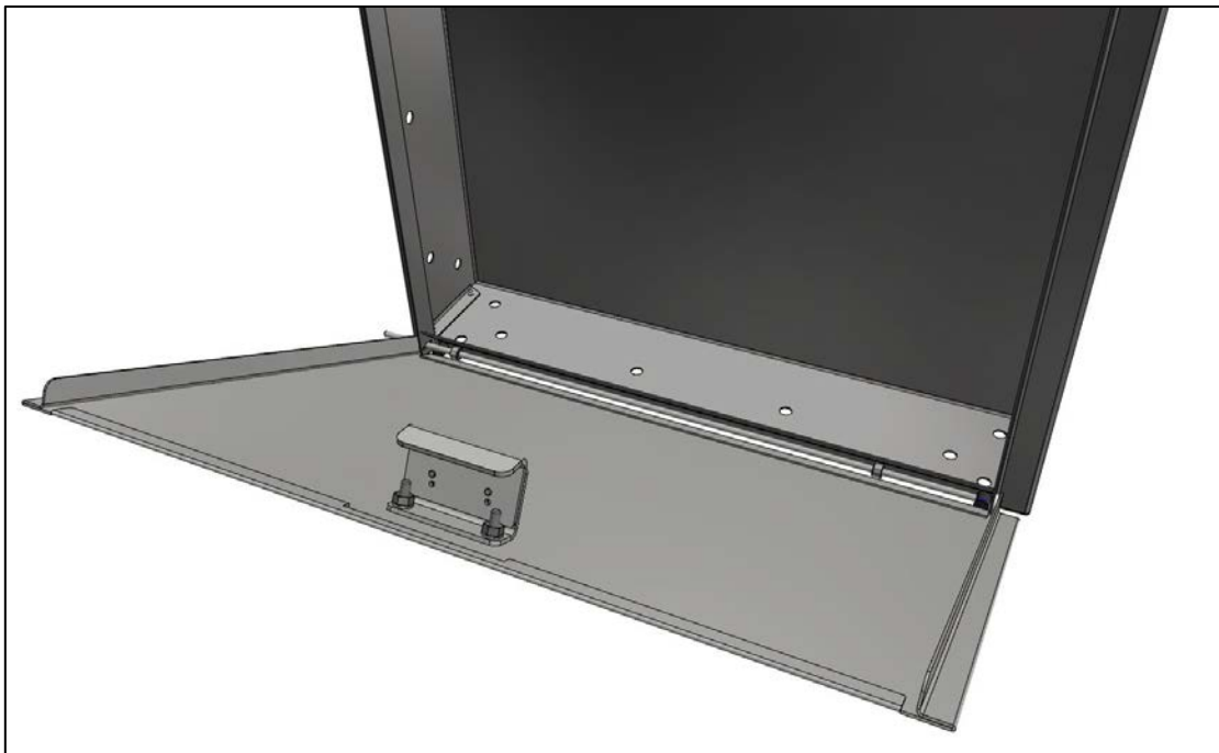
Fig. 58: Now push the axle with the two adjusting rings to the side so that one end of the axle hangs freely out of the box. ATTENTION: Pay attention to the spacer discs and their original positioning. These must be installed in exactly the same position during assembly
